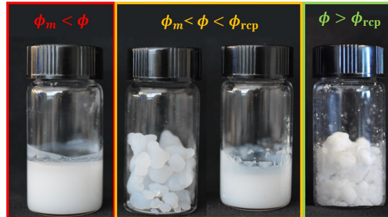
FIG. 3. Result of mixing suspensions of silica particles at different mass fractions \phi^{\text{wt}} . From left to right, the first vial corresponds to \phi^{\text{wt}} < \phi_m^{\text{wt}} with and without vibrations (here, \phi^{\text{wt}} = 23 wt% and vibrations are not applied). The second and third vials correspond to \phi_m^{\text{wt}} < \phi^{\text{wt}} < \phi_{\text{rcp}}^{\text{wt}} (here, \phi^{\text{wt}} = 29 wt%), without vibrations (second vial) or when vibrations are continuously applied during mixing (third vial). The last vial corresponds to \phi^{\text{wt}} > \phi_{\text{rcp}}^{\text{wt}} with and without vibrations (here, \phi^{\text{wt}} = 30 wt% and vibrations are applied). The studied suspension is characterized by \phi_m^{\text{wt}} \simeq 0.24 and \phi_{\text{rcp}}^{\text{wt}} \simeq 0.3 .
