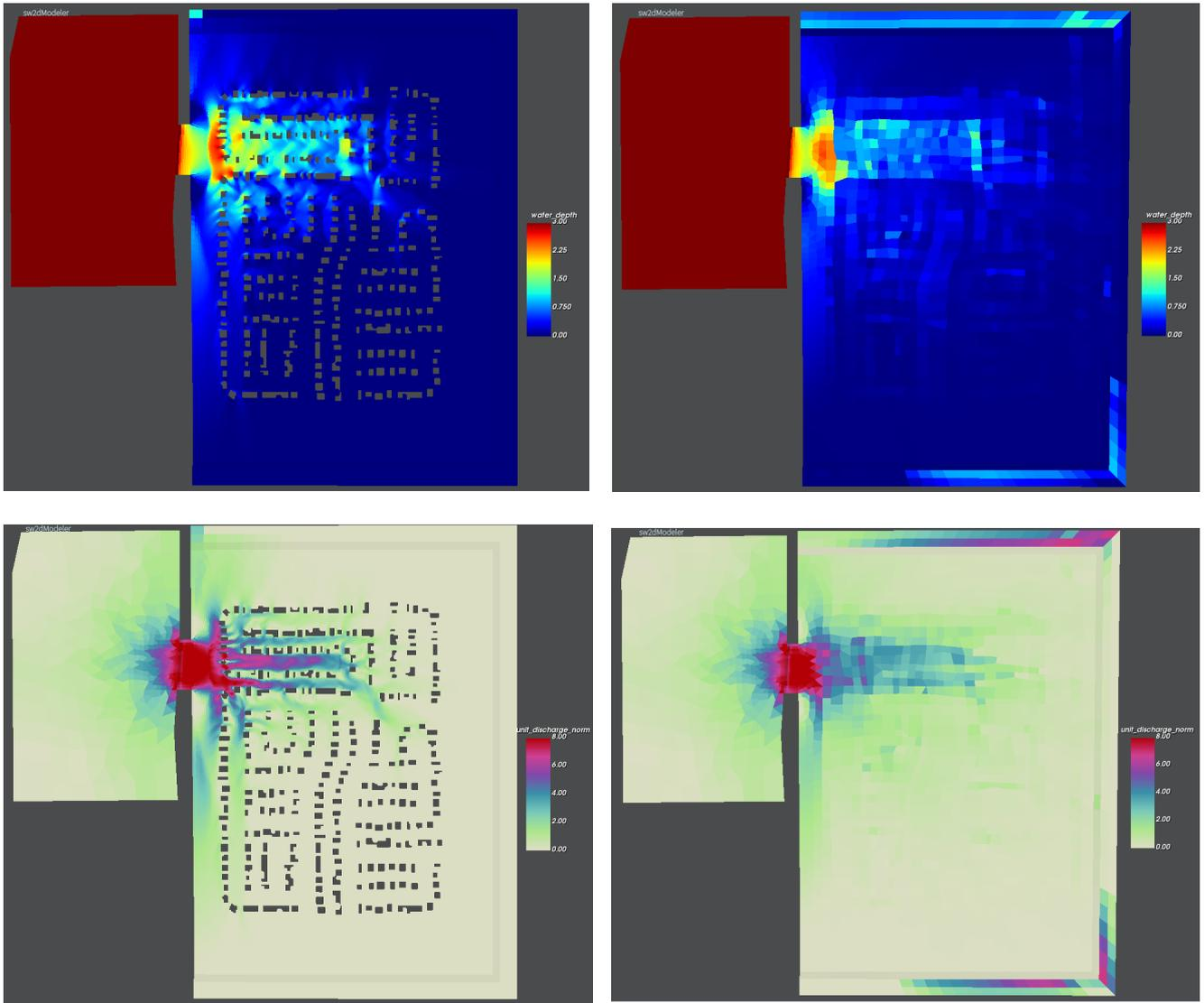
Figure 13: water depth (top row) and unit discharge norm (bottom row) at  $t = 120s$  for the SW (left column) and DIP (right column) simulations of the Sacramento test case. The color bars were adjusted for a better visualization of the solution within the neighbourhood. The water depth in the Water Channel is constant and equal to 8 m.
