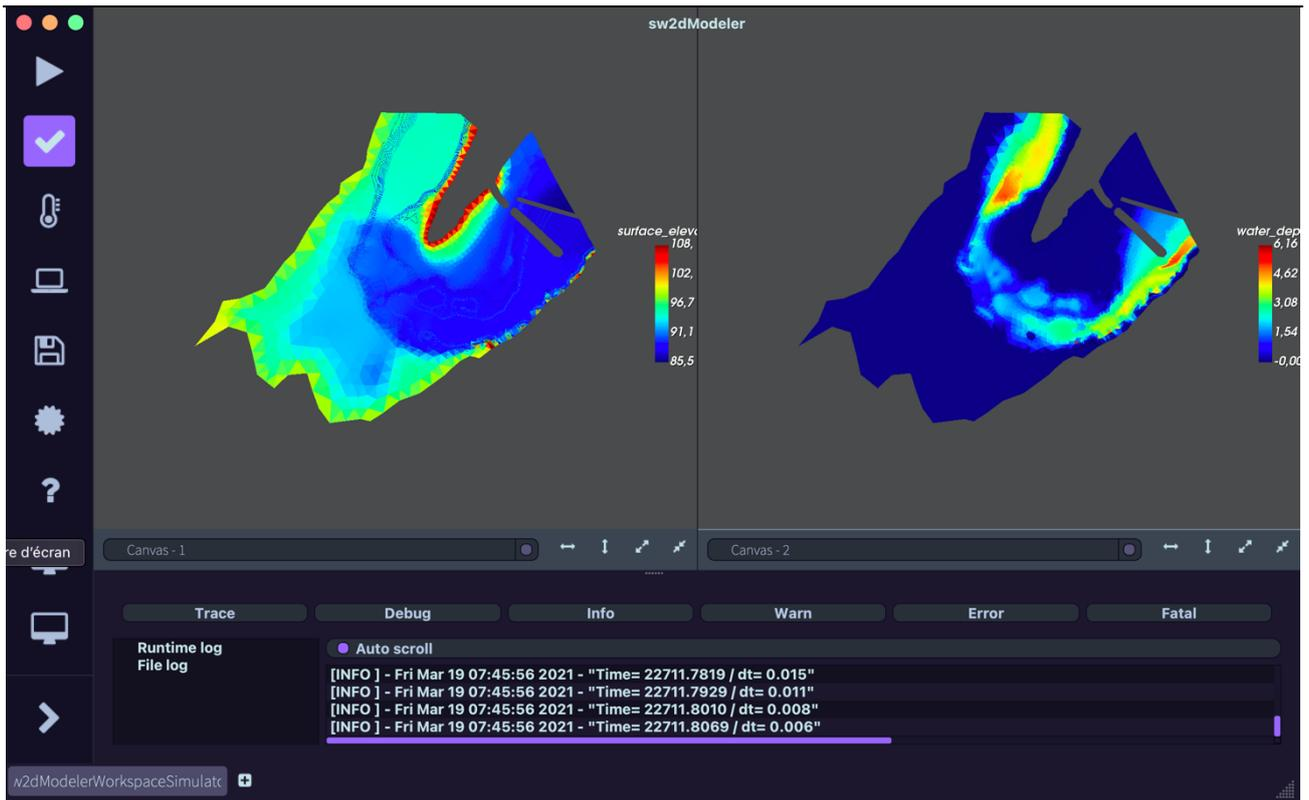
**Figure 9:** Visualization in the SW2D GUI of results obtained for Gardon test case near the beginning of the flood pic. Left: surface elevation (the ground elevation is displayed when there is no water in the cell). Right: water depth.
