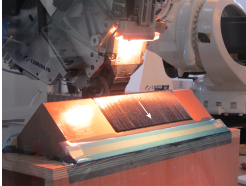
Fig. 2. AFP L-beam specimen production. the arrow indicates the direction of the fibres.
