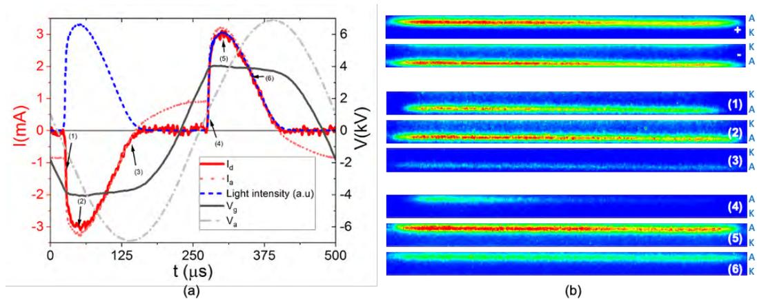
**Fig 1.** Homogeneous discharge in air at  $f=2\text{kHz}$  and  $V_{pp}=13.8\text{ kV}$ .  $I_a$  and  $I_d$  are the current applied to the DBD and the discharge current.  $V_g$  and  $V_a$  are the gas voltage and the applied voltage.
