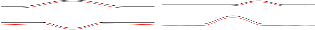
Figure 9: Reconstruction of two shape defects. In black, the initial shape of \Omega , and in red the reconstruction, slightly shifted for comparison purposes. In both cases, h = 0.1 , \omega_{\max} = 17 and the interval (0, \omega_{\max}) is discretize with 170 points. The relative L^2 -error is 4.7% on the left and 5.1% on the right. Functions g_1 and g_2 are given in (E5) and (E6).
