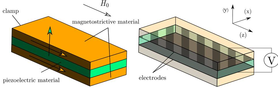
Figure 6: Diagram of the composite structure ( $3 \times 6 \times 14$  mm). For all simulations, it was discretized in  $12 \times 14 \times 28$  elements
