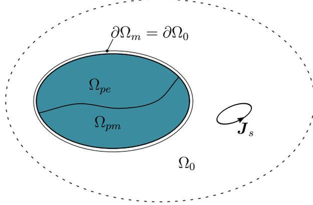
Figure 2: Subdomains of the magnetic problem based on a FEM-BEM formulation. The FEM is associated with the bounded domain  $\Omega_m = \Omega_{pe} \cup \Omega_{pm}$  and the BEM with the exterior infinite domain  $\Omega_0$  corresponding to an infinite free space. The FEM and BEM are coupled on the common boundary  $\partial\Omega_m$ .
