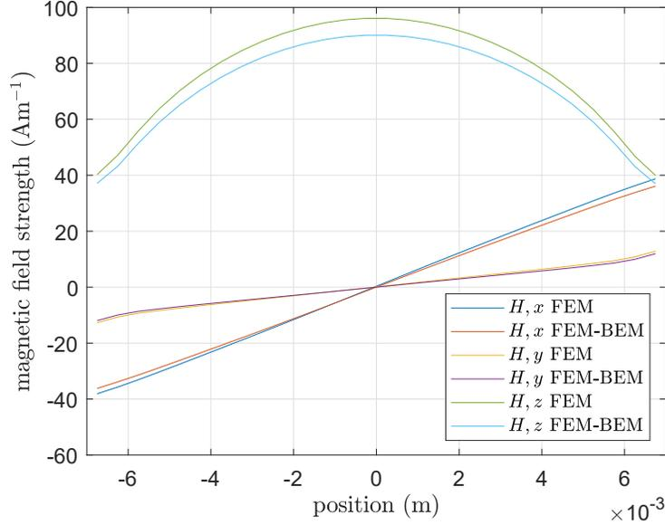
Figure 12: Comparison between the resulting magnetic field  $\mathbf{H}$  between the FEM 1 and FEM-BEM approaches along the (z) component of the position inside the magnetolectric device at its center.
