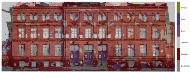
Figure 5. Result of the semantic segmentation on the test data superimposed on the original orthophoto.
