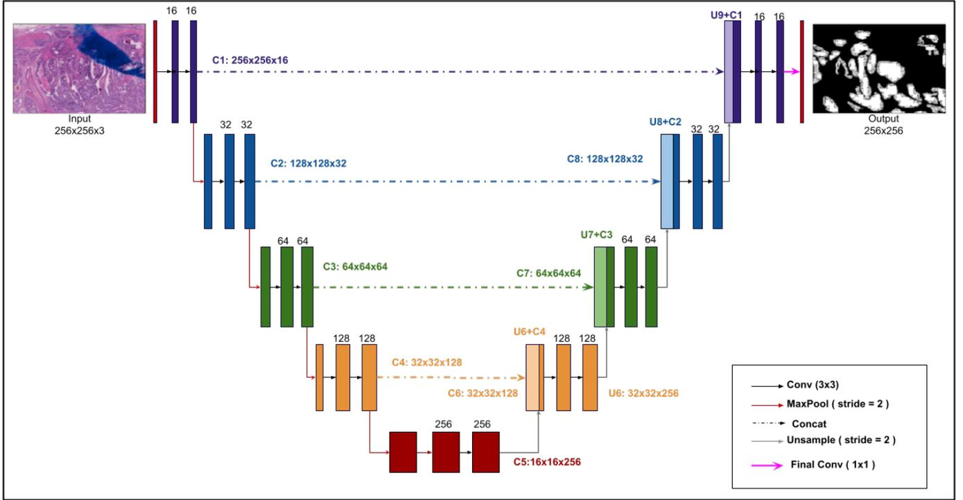
Figure 1: Architecture of the proposed UNET model.
