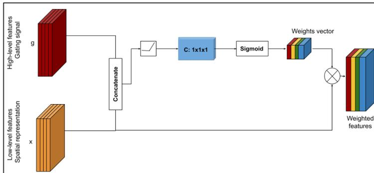
Figure 2: Attention mechanism: inside an attention Gate
