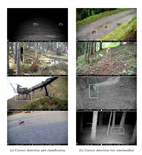
Figure 8: Examples of results of detection and classification (detection threshold on the bounding boxes confidence of 90%)
