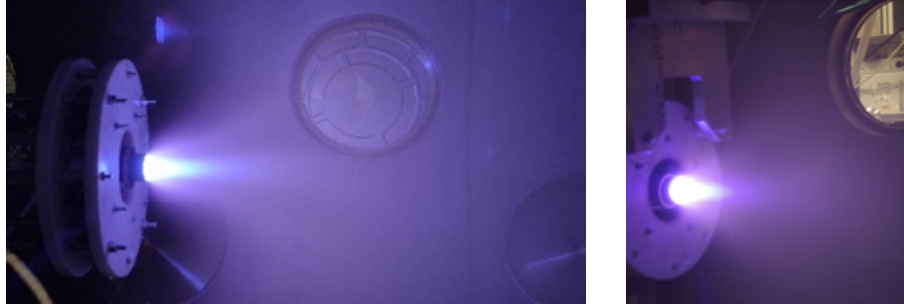
Fig. 7. TU-EBBM operating with Krypton on the thruster stand (left) and on the Thrust Balance (right) as part of the pre-test activities and the Coupling Test respectively.
