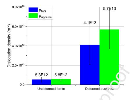
Figure 13: Representation of the dislocation density measured for two different grains: a nondeformed ferrite grain and a 3% deformed austenity grain. The measure of dislocation density obtained by clustering (in green) is compared with another measure (in blue) taken directly from the images, which consists of dividing the total numbe:  $N \neq i$  dislocations visible on the image by the surface of this image.
