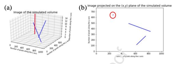
Figure 10:(a) Example of dislocation (in blue) obtained with a r ndo n direction in a three-dimensional volume and a red dislocation that is almost perpendicular to u = (X, Y) plane. The simulated volume is comparable to the experimentally explored volume. (b) From ted image of the volume on the (X,Y) plane with the dislocation almost perpendicular to the surface which appears as a point (red circle).
