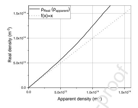
Figure 12: Representation of the real dislocation der sit, obtained in a three-dimensional volume, as a function of the apparent density obtained on a projected image of the volume. The divergence that appears comes from the phenomenon of over 1 app ing vislocations.
