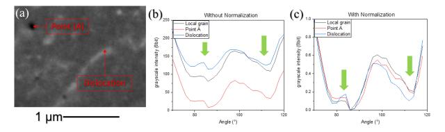
Figure 5: (a) BSE image of dislocation contained in an undeformed ferrite grain obtained at an accelerating voltage of 20 keV. (b) Intensity profile of the matrix (in black) of a dislocation pixel (in blue) and of a black point (in red) without normalization. The green arrows represent conditions where dislocations are visible in white on a black background. (c) The strate intensity profile as (b) with normalization.
