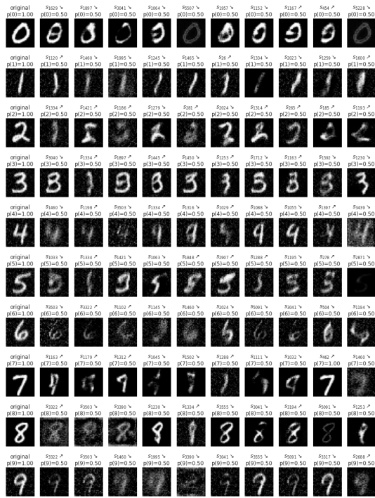
Figure 7: Illustration of corner cases found for each class. By starting from the average image in StyleSpace for the class, we manipulate its latent code in one of the top ten influential dimensions until the classifier shifts its prediction (softmax probability for the given class falls to 0.50). Above the images are displayed the StyleSpace dimension index, an arrow representing the direction to follow (augment or reduce the value), and the classifier output for the true class.
