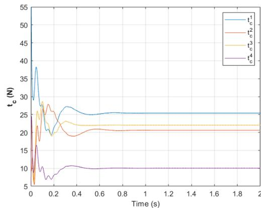
FIGURE 10 – Tension in the cables after a perturbation
