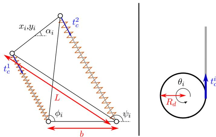
FIGURE 2 – Left : representation of the X-joint (in black) actuated by cables (in grey) in parallel with springs (in orange). Right : representation of the motor (in black) pulling the cable (in grey) through a winch
