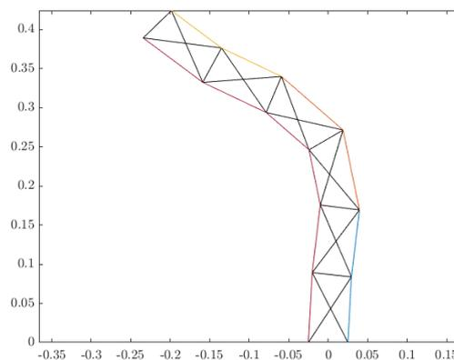
FIGURE 1 – Schematic of a tensegrity robot with 6 X-joints (black) and 4 cables (purple, blue, red, yellow).
