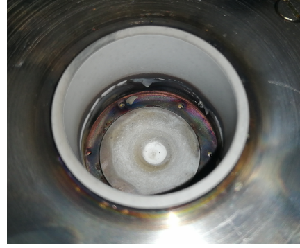
Fig. 4 Eroded central ceramic
