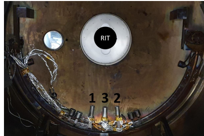
Fig. 2 Experimental apparatus used at ESTEC in the GIGANT chamber. Location 1 and 2 are \pm 7.2^\circ off-centre. Probe are located 63 cm from the rotation axis of the arm. The latter is 30 cm upwards the thruster exit plane.
