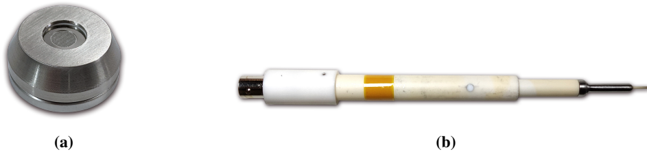
Fig. 3 (a) Retarding potential analyzer and (b) RF-compensated Langmuir probe.
