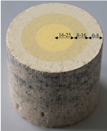
Figure 3: View of a CRA specimen showing the three slices used for determination of water content (0-8 mm; 8-16 mm and 16-25 mm)
