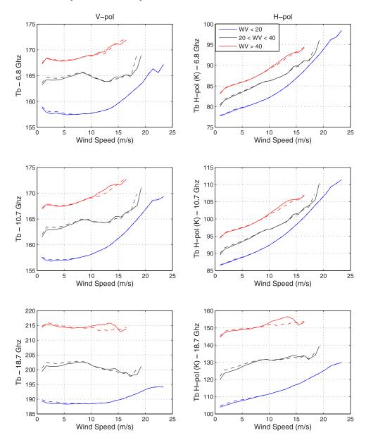
**Figure 6.** Mean V-pol (left panels) and H-pol (right panels) Tb's binned as a function of ECMWF wind speed (m/s), at 6.8 GHz (top), 10.7 GHz (middle), and 18.7 GHz (bottom), and for different integrated water vapor ranges: 0 mm < WV < 20 mm (blue lines), 20 mm < WV < 40 mm (black lines), and 40 mm < WV < 60 mm (red lines). WindSat (dashed lines) and Jason microwave radiometer (dashed lines) integrated water vapor data are used.
