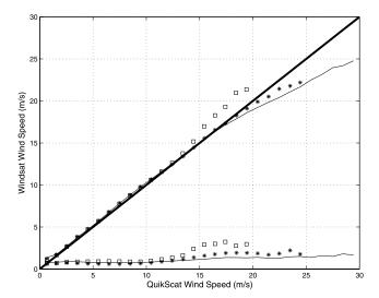
**Figure 14.** Mean WindSat speeds binned by QuikSCAT wind speeds, for 0 mm < WV < 20 mm (solid lines), 20 mm < WV < 40 mm (star), and 40 mm < WV < 80 mm (squares). The thick solid line is the perfect fit line. The bottom curves display the standard deviation of the WindSat minus QuikSCAT differences. WV stands for the WindSat integrated water vapor content. Each bin contains at least 50 collocated measurements.
