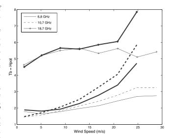
**Figure 8.** H-pol Tbs standard deviations binned as a function of QuikSCAT (thin lines) and NCEP (thick lines) wind speed (2 m/s bins), at 6.8 GHz (solid lines), 10.7 GHz (dashed lines), and 18.7 GHz (crosses). The integrated water vapor range is 0 mm < WV < 20 mm.
