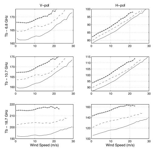
**Figure 7.** Mean V-pol (left panels) and H-pol (right panels) Tb's binned as a function of QuikSCAT wind speed (m/s), at 6.8 GHz (top), 10.7 GHz (middle), and 18.7 GHz (bottom), and for different integrated water vapor ranges: 0 mm < WV < 20 mm (solid lines), 20 mm < WV < 40 mm (dashed lines), and 40 mm < WV < 60 mm (plus signs). WindSat integrated water vapor data are used.
