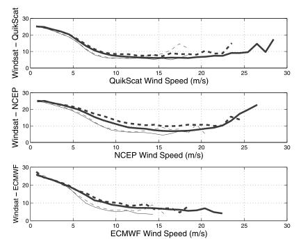
**Figure 16.** Standard deviation (degrees) of the WindSat wind direction minus QuikSCAT (top panel), NCEP (middle panel), ECMWF (bottom panel) wind direction, as a function of wind speed in tropical (thin lines) and midlatitude areas (thick lines). WV ranges are 0 mm < WV < 20 mm (solid lines) and 20 mm < WV < 80 mm (dashed lines). A minimum of 50 data points is required in each 1 m/s bin.
