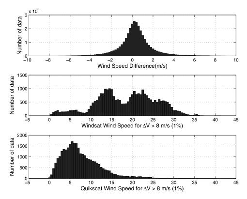
**Figure 13.** WindSat minus QuikSCAT wind speed difference distribution (top panel), WindSat (middle panel) and QuikSCAT (bottom panel) wind speed distribution for wind speed differences greater than 8 m/s.
