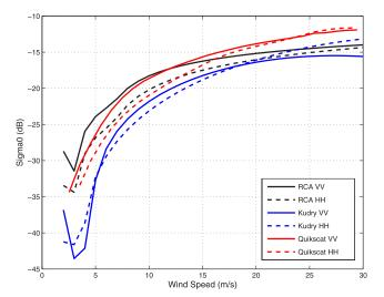
**Figure 4.** Mean Ku-band VV (solid lines) and HH (dashed lines)  $\sigma_0$  (dB) computed with the RCA model (black), the Kudryavtsev model (blue), and the QuikSCAT data (red), as a function of wind speed (m/s).
