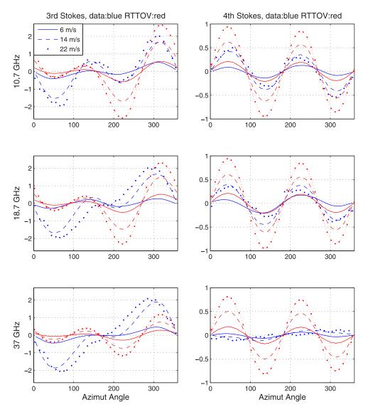
**Figure 12.** Mean 3rd (left panels) and 4th (right panels) Stokes parameters for WindSat (blue lines) and RTTOV-8 model (red lines) binned as a function of the relative wind direction (degrees), at 10.7 GHz (top), 18.7 GHz (middle), and 37.0 GHz (bottom), and for different wind speed ranges: 4 m/s < WS < 8 m/s (solid lines), 12 m/s < WS < 16 m/s (dashed lines), 20 m/s < WS < 24 m/s (dotted lines).
