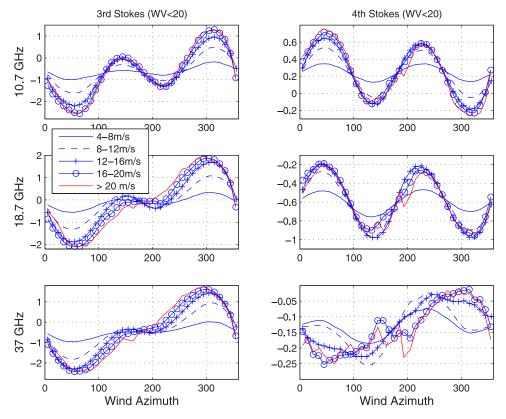
**Figure 10.** Mean 3rd (left panels) and 4th (right panels) Stokes parameters binned as a function of the relative wind direction (degrees), at 10.7 GHz (top), 18.7 GHz (middle), and 37.0 GHz (bottom), and for different wind speed ranges: 4 m/s < WS < 8 m/s (solid lines), 8 m/s < WS < 12 m/s (dashed lines), 12 m/s < WS < 16 m/s (+), 16 m/s < WS < 20 m/s (o), WS > 20 m/s (red lines). Integrated water vapor is taken in the range WV < 20 mm.
