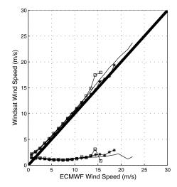
**Figure 15.** Mean WindSat speeds binned by Jason winds (left) and ECMWF winds (right), for 0 mm < WV < 20 mm (solid lines), 20 mm < WV < 40 mm (star signs), and 40 mm < WV < 80 mm (square signs). The thick solid line is the perfect fit line. The bottom curves display the standard deviation of the WindSat minus Jason (left) and ECMWF (right) differences. WV is retrieved from the Jason JMR radiometer. Each bin contains at least 20 points.
