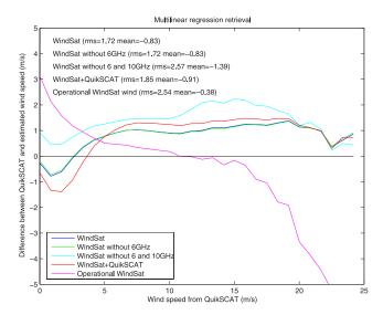
**Figure 18.** Wind speed errors for different combinations of observations, stratified by the QuikSCAT wind speed taken as a reference. For each combination, the RMS and mean errors calculated over the original data set (including rainy pixels) are indicated.
