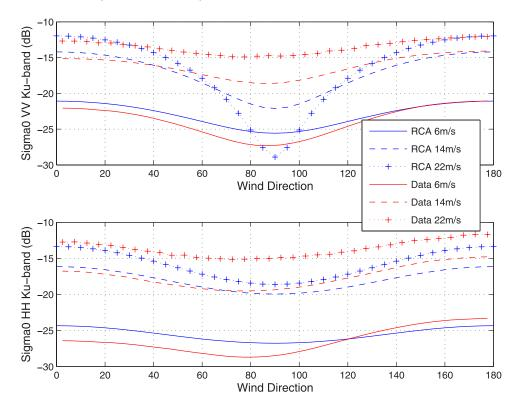
**Figure 5.** Mean Ku-band VV (top panel) and HH (bottom panel)  $\sigma_0$  (dB) computed with the RCA model (blue) and QuikSCAT data (red), as a function of the wind direction (degrees), for 6 m/s (solid lines), 14 m/s (dashed lines), and 22 m/s (+) mean wind speed.
