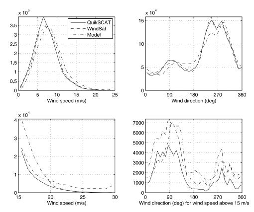
**Figure 3.** Distribution of the wind speeds from the collocated database. Histograms are presented for OuikSCAT, WindSat, and the NCEP model estimates.
