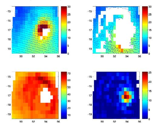
**Figure 17.** QuikSCAT (top left) and WindSat (top right) wind fields, speed in m/s, for non rainy areas, in a tropical storm, February 10, 2003, 12h00 UTC. WindSat integrated water vapor content (bottom left in mm) and rain rate (bottom right in mm/hr).
