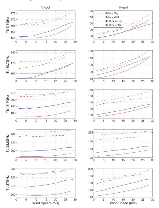
**Figure 9.** Mean V (left panels) and H (right panels) Tb's binned as a function of QuikSCAT wind speed (m/s), at 6.8 GHz, 10.7 GHz, 18.7 GHz, 23.8 GHz, and 37.0 GHz, respectively from top to bottom, for a dry atmosphere: 0 mm < WV < 20 mm (solid lines), and for a wet atmosphere 20 mm < WV < 60 mm (dashed lines). WindSat data are plotted as blue lines and RTTOV model as red lines.
