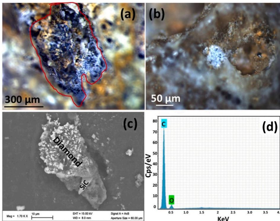
**Fig. 2.** Porosities of siliceous rock a) Binocular images of siliceous rock porosities, b) Optical images of diamond present in porosities, c) SEM image of a cluster of diamonds bearing SiC extracted from porosities and d) EDS spectrum of diamond.
