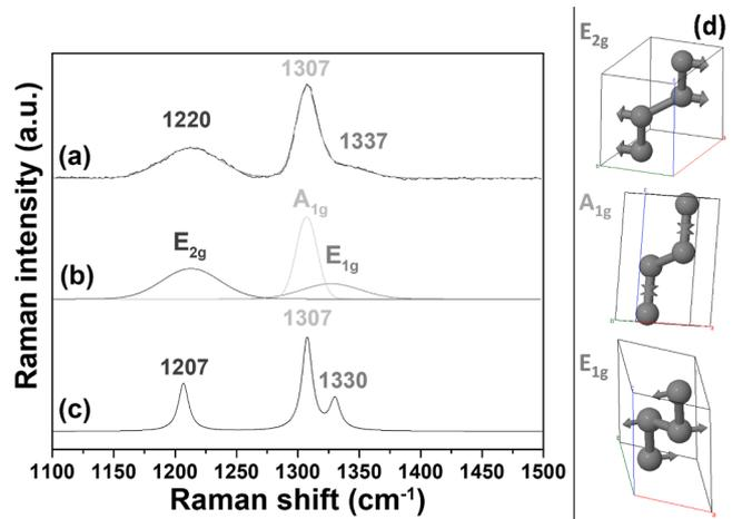
**Fig. 4.** (a) Experimental Raman spectrum of lonsdaleite (b) The active vibrational modes  $E_{1g}$ ,  $A_{1g}$  and  $E_{2g}$  obtained via deconvolution of the Raman experimental spectrum, (c) Theoretical Raman spectrum of lonsdaleite with Gaussian line shape and a FWHM of 10  $\text{cm}^{-1}$  and (d) The presentation of the Raman vibration modes of lonsdaleite.
