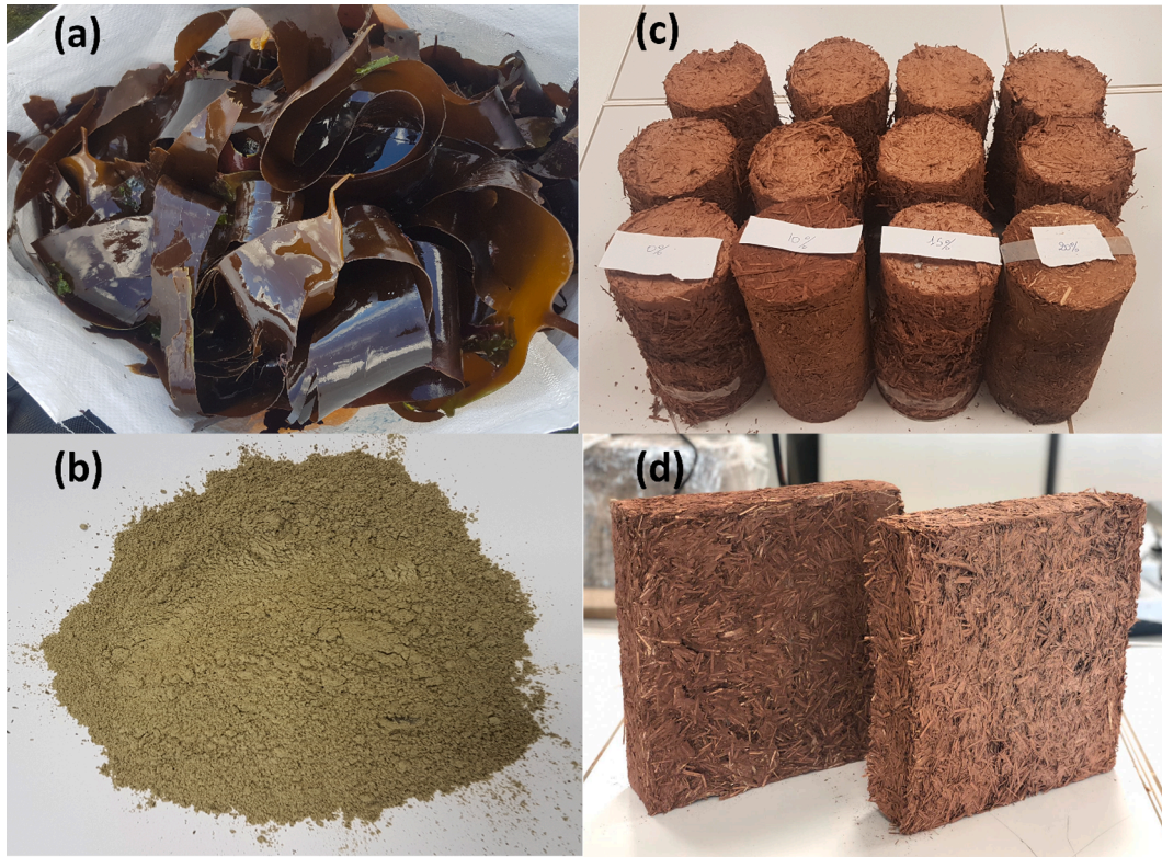
Fig. 1. (a) Raw Laminaria digitata . (b) Laminaria digitata powder used as earth substitution. (c) Samples used for mechanical tests ( \varnothing 11 cm \times 22 cm) and (d) samples used for thermal analysis ( 30 \times 30 \times 4 cm 3 ).
