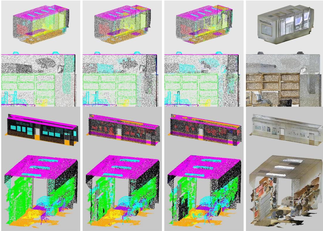
Fig. 9. Semantic segmentation tests results obtained after training with synthetic data sampled with VLS, from left to right : truth, colored synthetic data, colorless synthetic data, raw scene.
