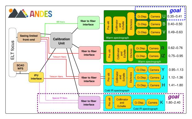
Figure 3. ANDES architectural design, outlining the instrument subsystems: Front End (seeing-limited and AO assisted with SCAO unit), Fibre Link, Calibration Unit, VIS-Blue, VIS-Red, NIR and NIR-K (cold spectrographs). Andes Logo by Alexis Lavail (Uppsala).
