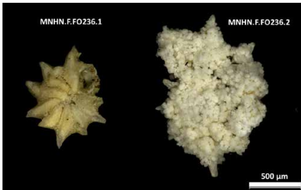
Figure 1. Two specimens of the foraminifer CNECTK B. On the left, the specimen is in a fair condition. On the right, the specimen is severely damaged by calcium formate crystalline growth ©MNHN
