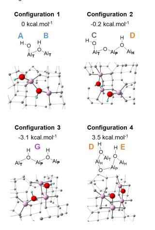
Figure 6. Calculated hydroxyl group configurations and their relative energies, for the partially hydroxylated (110) surface of  $\gamma$ -alumina with  $\theta$  = 0.7 OH/nm<sup>2</sup>.
