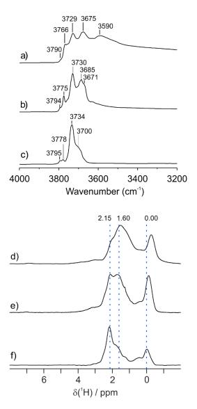
Figure 1. Comparison of spectra for several  $\gamma$ -aluminas: DRIFTS spectra in the hydroxyl stretching region, for (a) Al<sub>2</sub>O<sub>3-300</sub>, (b) Al<sub>2</sub>O<sub>3-500</sub>, and (c) Al<sub>2</sub>O<sub>3-700</sub>, as well as <sup>1</sup>H MAS NMR spectra (18.8 T, spinning frequency 20 kHz), for: (d) Al<sub>2</sub>O<sub>3-300</sub>, (e) Al<sub>2</sub>O<sub>3-500</sub>, and (f) Al<sub>2</sub>O<sub>3-700</sub>.
