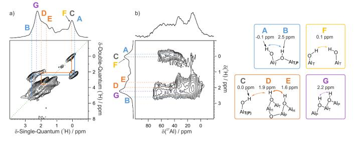
Figure 2. (a) <sup>1</sup>H-<sup>1</sup>H DQSQ MAS NMR spectrum, and (b) <sup>1</sup>H-<sup>27</sup>Al D-HMQC MAS NMR spectrum, for  $Al_2O_{3-700}$  (18.8 T, spinning speed 20 kHz), and the hydroxyl environments deduced from the correlations, with their associated <sup>1</sup>H NMR chemical shifts
