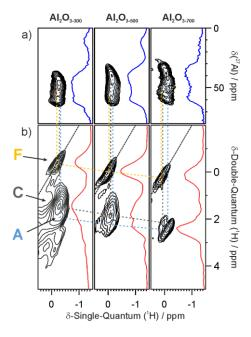
**Figure 4.** Comparison in the region of the terminal hydroxyl group signals, of (a) <sup>1</sup>H-<sup>1</sup>H DQ-SQ NMR spectra, and (b) <sup>1</sup>H-<sup>27</sup>Al D-HMQC MAS NMR spectra (18.8 T, spinning speed 20 kHz) for Al<sub>2</sub>O<sub>3-300</sub>, Al<sub>2</sub>O<sub>3-500</sub> and Al<sub>2</sub>O<sub>3-700</sub>, as well as the corresponding projections in the indirect dimension (red and blue traces).
