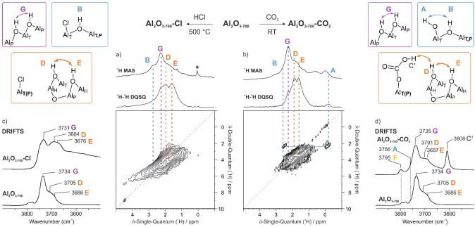
Figure 3. <sup>1</sup>H MAS NMR and <sup>1</sup>H -<sup>1</sup>H DQSQ MAS NMR spectra of (a) Al<sub>2</sub>O<sub>3-700</sub>-CI, and (b) Al<sub>2</sub>O<sub>3-700</sub>-CO<sub>2</sub> (18.8 T, spinning speed 20 kHz; \* : impurity, not present in the 2D spectrum), and their corresponding IR spectra (c, d, arbitrary intensity scale). Proposed structures for various hydroxyl-bearing Al sites present after reaction are also shown.
