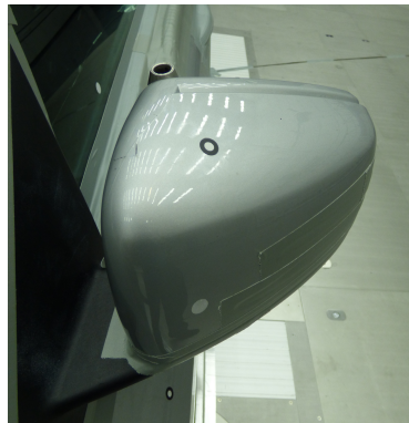
Fig. 9 - Omnidirectional source placed near the rear-view mirror.
