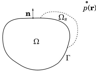
**Fig. 1** - FW-H schematic set up.  $\Omega$  and  $\Gamma$  denote the interior and the boundary of the structure, while  $\Omega_s$  accounts for the source area. The pressure at the observer point  $\mathbf{r}$  can be obtained from the source region only.
