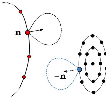
**Fig. 4** - Reciprocity principle applied to dipolar FRFs. The computation of a half dipole on the mesh radiating toward a microphone can be traded against the one of a dipole with opposite direction located on the array toward the surface.
