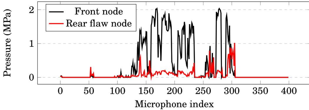
**Fig. 11** - *FRF amplitude between two specific nodes and the 400 microphones at  $f = 3000$  Hz.*
