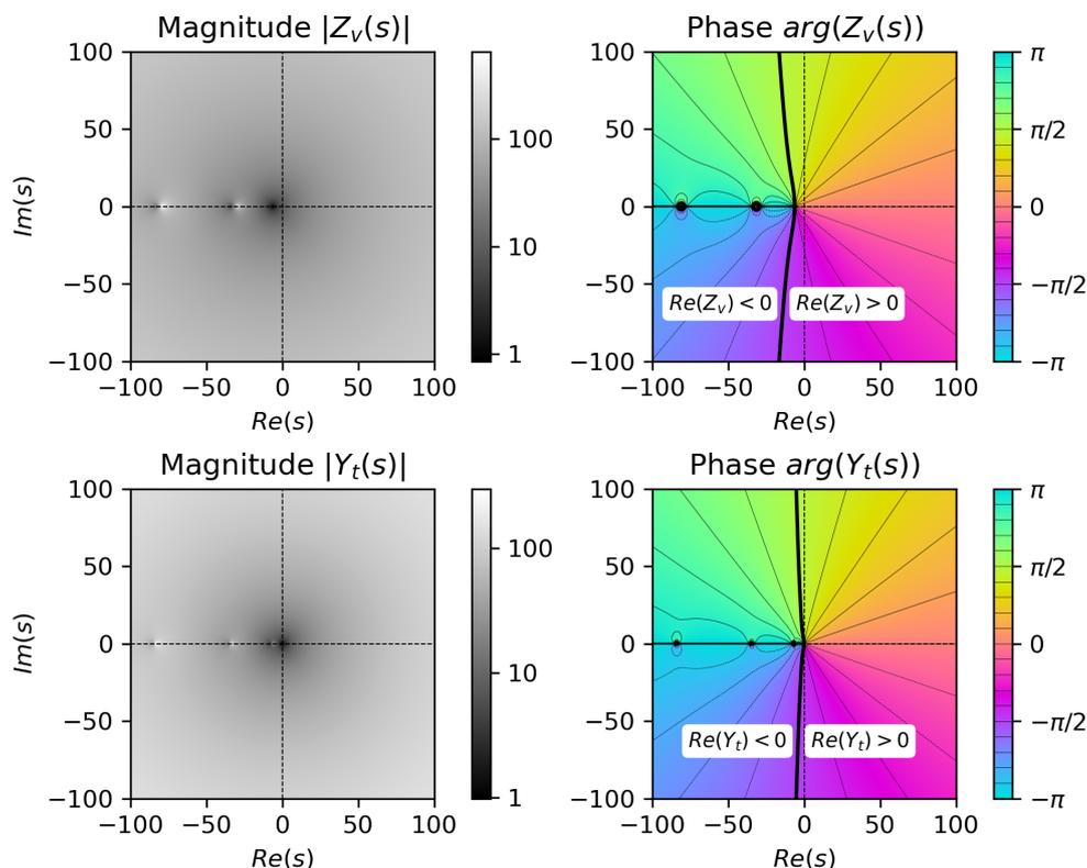
Figure A.7: Amplitude (left) and phase (right) of the analytic extension to the complex plane of the **lineic immittances**  $Z_v$  (top) and  $Y_t$  (bottom) defined by equation (2). The loss coefficients (54) have been calculated for a cone with angle  $\Theta = \pi/4$ . The calculation uses unitary coefficients  $R = \text{Pr} = \rho_0 = \mu = 1$ . Black curves on the phase plots indicate the locus of points where the real part of the **lineic immittances** is zero.
