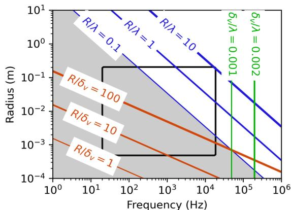
Figure 2: Range of validity of the low reduced frequency model (grayed), compared to the range of tube radii and frequencies of interest in musical acoustics (rectangle). Iso-lines of the ratios of radius  $R$ , wavelength  $\lambda$  and boundary layer thickness  $\delta_v$  are shown. The low reduced frequency model assumes  $R \ll \lambda$  and  $\delta_v \ll \lambda$ , but does not assume  $R \gg \delta_v$ .
