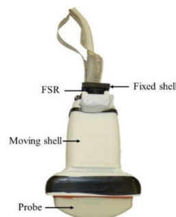
Figure 4. Instrumented probe—Force measurement.
