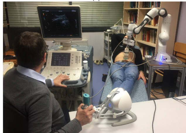
Figure 6. (a) Tele-operation chain using a 6-degrees-of-freedom (DoF) master device and a 7-DoF collaborative slave robot; (b) Doppler ultrasound test performed by the angiologist using the tele-operation platform.
