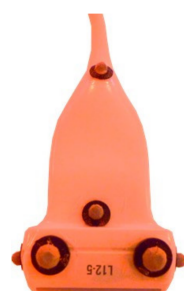
Figure 2. Reflective markers on probe.
