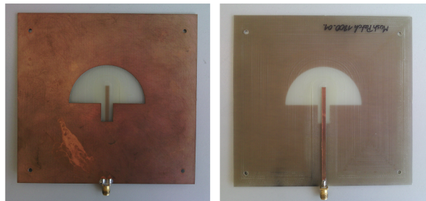
Fig. 2. Picture of the wideband slot-based antenna under test: top view (left) and bottom view (right).
