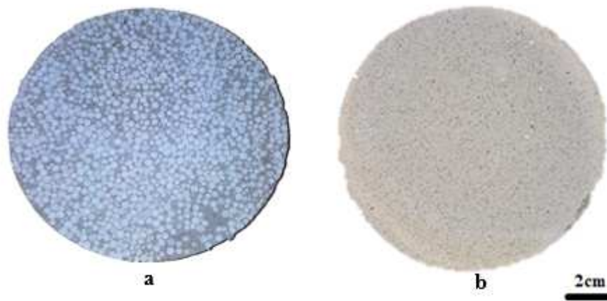
148 Fig.1. a) Expanded polystyrene mortar; b) Cement paste
