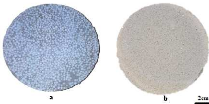
Fig.1. a) Expanded polystyrene mortar; b) Cement paste
