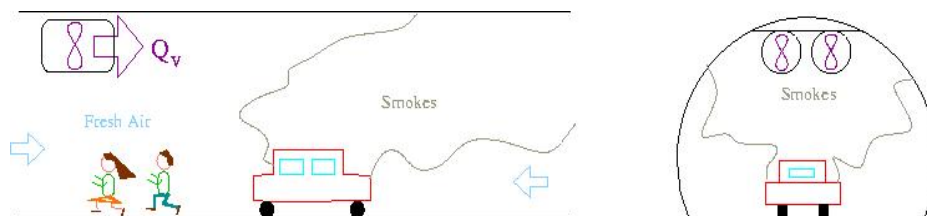
Fig 1 . Longitudinal ventilation strategy
