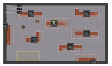
Fig. 4: Overview of a  $6 \times 6$  job shop scenario in *Gobot-Sim* composed of one *input* machine (on the left) that feeds the environment with unprocessed packages, six *processing* machines that can do a predefined process, and one *output* machine (at the bottom right) that receives fully processed packages. Two robots can be used to dispatch packages on the machines. The recharge area (in yellow) is available at the bottom.
