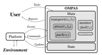
Fig. 2: A high-level view of the operation and architecture of OMPAS. The *user*, either an operator or a program, can send new tasks to be executed. A new task is processed by the *main* thread, which creates a new thread to handle the execution of the task. The user receives task status reports and platform status updates.
