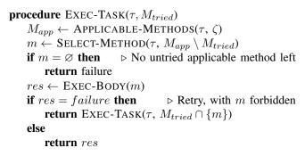
Fig. 3: Adaptation of RAE's procedure for executing a task  $\tau$ . The procedure arbitrarily selects a method m that is applicable in the current state  $\zeta$  and has not been previously tried.
