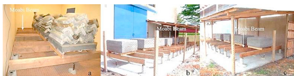
Fig. 1. a) Air-conditioned environment. b) Unsheltered environment. c) Sheltered environment
