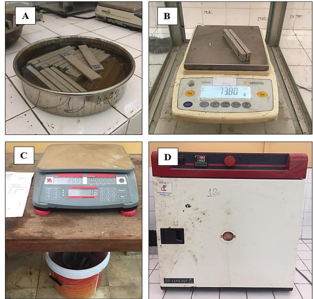
Fig. 4. (a) keep specimens saturated, (b) weighting them on electronic scale, (c) water immersed weighting, and (d) drying the specimens by microwave
