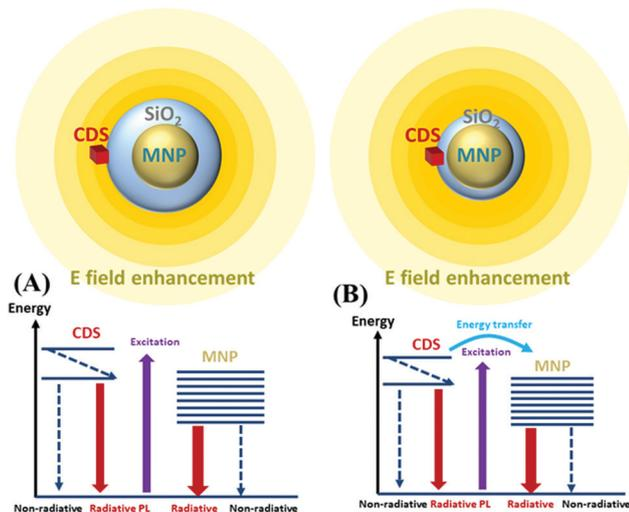
**Scheme 3** Representation of the donor-acceptor system with the excitation and emission processes of the CDS-MNP surface hybrid system. (A) a large shell thickness and (B) a short shell thickness are shown.
