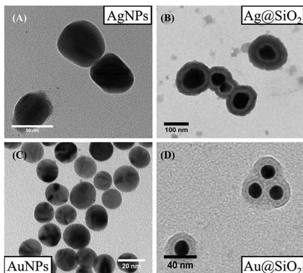
Fig. 4 Bright field TEM images of MNPs. (A) AgNPs; (B) Ag@SiO<sub>2</sub>; (C) AuNPs; (D) Au@SiO<sub>2</sub>.
