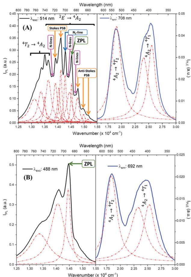
Fig. 5 PL (black) and PLE (blue) spectra of (A) ZAOC and (B) MAOC. The red-dashed lines represent Lorentzian fits. The green arrow indicates the zero-phonon line, the blue arrow indicates the N<sub>2</sub>-line, and the orange arrows indicate Stokes and anti-Stokes phonon sidebands (PSB). The pink arrows indicate different N-lines that appear when the concentration of Cr<sup>3+</sup> is ~0.2 mol%.
