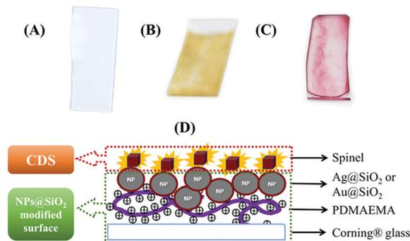
**Scheme 2** Surface modification schemes. (A) Cleaned Corning® glass; (B) Ag@SiO<sub>2</sub>; (C) Au@SiO<sub>2</sub>; (D) Scheme describing the ensemble formed with deposited spinels and MNPs-modified surfaces.
