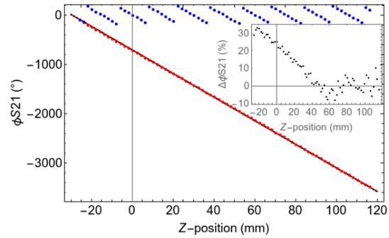
Fig. 6. Phase of the E-field as a function of the distance to the antenna ( $Z = 0$  corresponds to the aperture plane). Blue and red dots correspond to the raw data and to the unwrapped phase, respectively. The red line is a linear fitting curve. Dashed black line is the theoretical line. The inset indicates the relative error between measurement and fit as a function of the distance.
