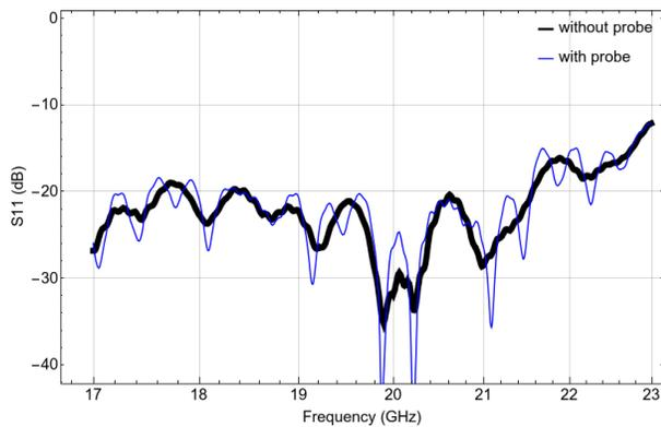
Fig. 2. Reflection coefficient of the antenna. Black curve:  $S_{11}$  of the antenna without the EO probe (reference). Blue curve:  $S_{11}$  of the antenna with EO probe placed in the reactive region (within the horn, in the vicinity of the apex).
