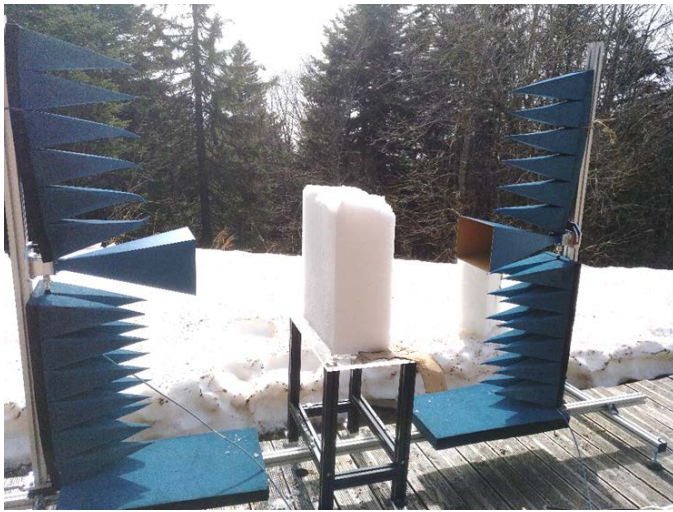
Fig. 3. Portable complex permittivity measurement bench.
