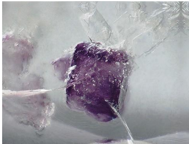
Figure 12. Purple fluorite cube, identified by micro-Raman spectroscopy, in a hyalite. Photomicrograph by U. Hennebois; field of view 1.2 mm.
