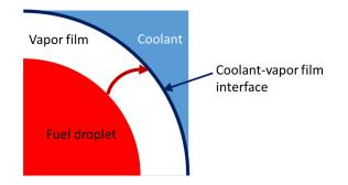
Fig. 6. Model of the heat exchange from the fuel droplet to the interface between the coolant and the vapor film, (red arrow).
