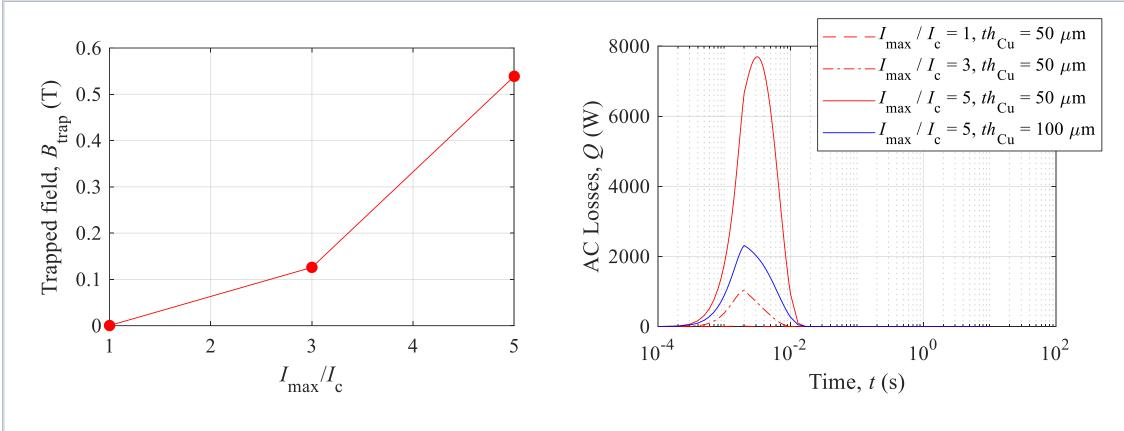
A compromise to be found between the losses, the copper section and the trapped field
