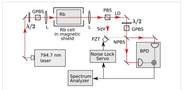
Figure 5. Figure of a polarization self-rotation set-up. SqV is the squeezed vacuum field. LO is the local oscillator. NPBS is a non-polarizing beamsplitter and GPBS is a Glan polarizing beamsplitter. BPD is a balanced photodiode detector. PZT is a piezo-electric translation actuator on a mirror. Reprinted with permission from [24]. © The Optical Society.
