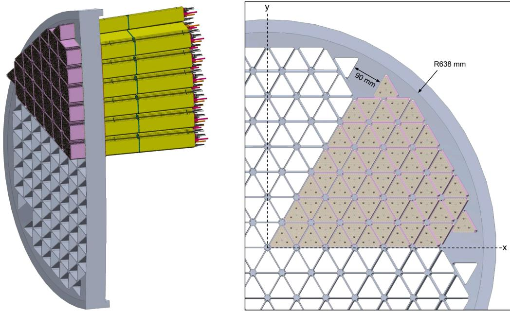
Figure 7: Focal plane layout for 348 fiber robot rafts (with 26,100 robots) on the MegaMapper per focal plane.
