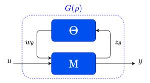
Fig. 3: Linear fractional representation of a parameter-varying system
