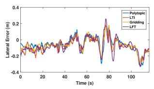
Fig. 23: Experimental lateral error of the LTI and LPV controllers (m)
