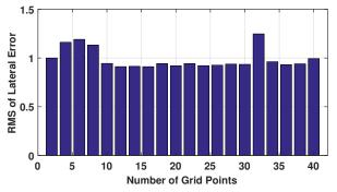
Fig. 15: Normalized RMS of the lateral error with respect to different number of gridding points  $n_q$
