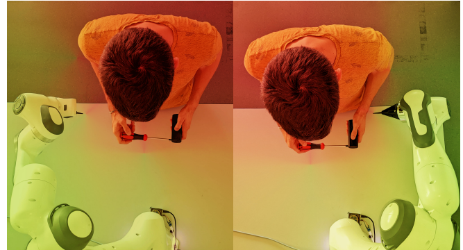
Fig. 1. A safe workspaces in a collaborative environment cannot be defined with static zones as it depends on the robot-operator states and tasks.
