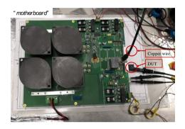
Fig. 1. Secure SC test-bench: max 600V, 400A, 100µs, 125°C.
