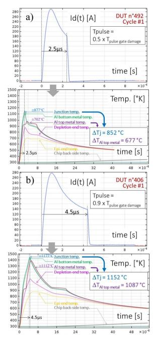
Fig. 3. Transient thermal simulation in short-circuit stress, a) Shortest pulse 2.5 $\mu$ s, b) Longest pulse 4.5 $\mu$ s. @V<sub>DS</sub> = 600V, V<sub>Drv</sub> = -5V/+18V, R<sub>Gate</sub> = 47\Omega, T<sub>Case</sub> = T<sub>Amb</sub>
