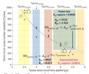
Fig. 6. Nb<sub>cycles</sub>( $T_{Pulse GD \%}$ ) fitting laws and parameters @V<sub>DS</sub> = 600V, V<sub>Drv</sub> = -5V/+18V, R<sub>Gate</sub> = 47 $\Omega$ .
