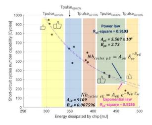
Fig. 7.  $Nb_{cycles}(E_{sc})$  fitting laws and parameters @V<sub>DS</sub> = 600V, V<sub>Drv</sub> = -5V/+18V, R<sub>Gate</sub> = 47 $\Omega$ .
