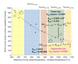
Fig. 8. Nb<sub>cycles</sub>( $\Delta T_{Al\_Top\_Metal}$ ) fitting laws and parameters @V<sub>DS</sub> = 600V, V<sub>Drv</sub> = -5V/+18V, R<sub>Gate</sub> = 47 $\Omega$ .
