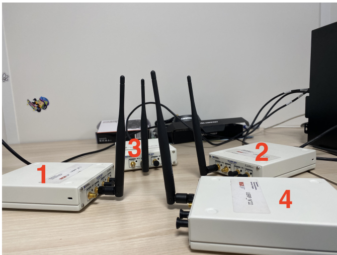
Fig. 5: Testbed setup using four USRPs.
