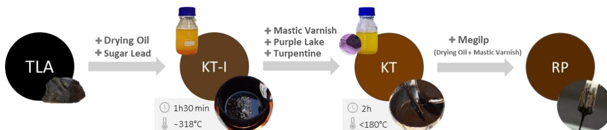
Figure 2: Schematic showing the sequence of samples taken during the production of W&N’s Bitumen Brown oil paint with the time and temperatures reached.
