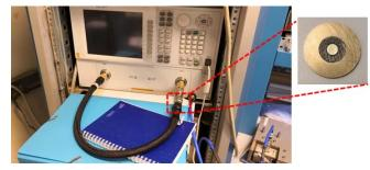
Fig. 2. Measurement for complex permittivity measurement 1MHz-18GHz
