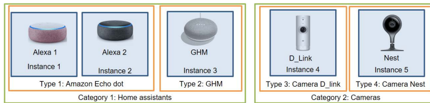
FIGURE 9. IoT devices classification levels. IoT devices can be classified at different levels of granularity: i) category, ii) type, and iii) instance. In this example, home assistants and cameras are two different categories of IoT devices. GHM (Google Home Mini) and Amazon Echo Dot are two types of Home assistants . Finally, Alexa 1 and Alexa 2 , are two instances of the Amazon Echo Dot .
